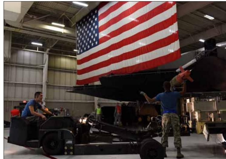
Left: Members of the 13th Aircraft Maintenance Unit transfer a GBU-38 using a MHU-83 "jammer" during the fourth quarter load competition at Whiteman Air Force Base, Mo., Jan. 6, 2017. The weapons load crew 4-member is responsible for operating the MHU-83 to safely transfer the GBU-38 to the aircraft in a timely manner.
